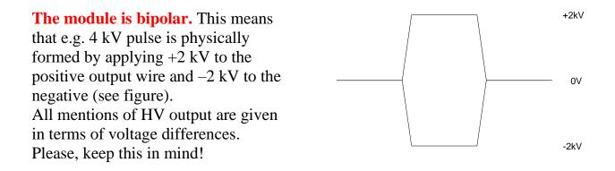
The modules require +24 V DC power supply and pulse generator to set an operating frequency and pulse width. An output voltage level can be programmed in working range by user either manually (through onboard configuration trimpot) or remotely (applying a DC voltage to the respective pin).
