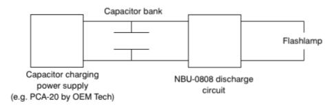
By default, NBU-0808 includes capabilities both for serial and external triggering (See *Triggering* section for details). Simplified as well as more complex modifications are available on request.
