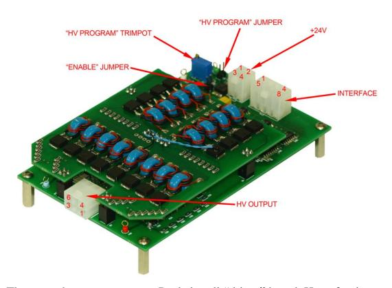
There are three connectors at Pockels cell "driver" board. Hereafter is description of corresponded female connectors (supplied with the board)
