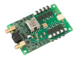
On request we can build QBY-BT driver based on QBU-nano board of any available modification. Advantages are even faster rise and fall times, a shorter pulse width and higher output voltages. The main disadvantage is a pulse repetition rate limited with 0.5-2kHz max. Please contact us for this option.
